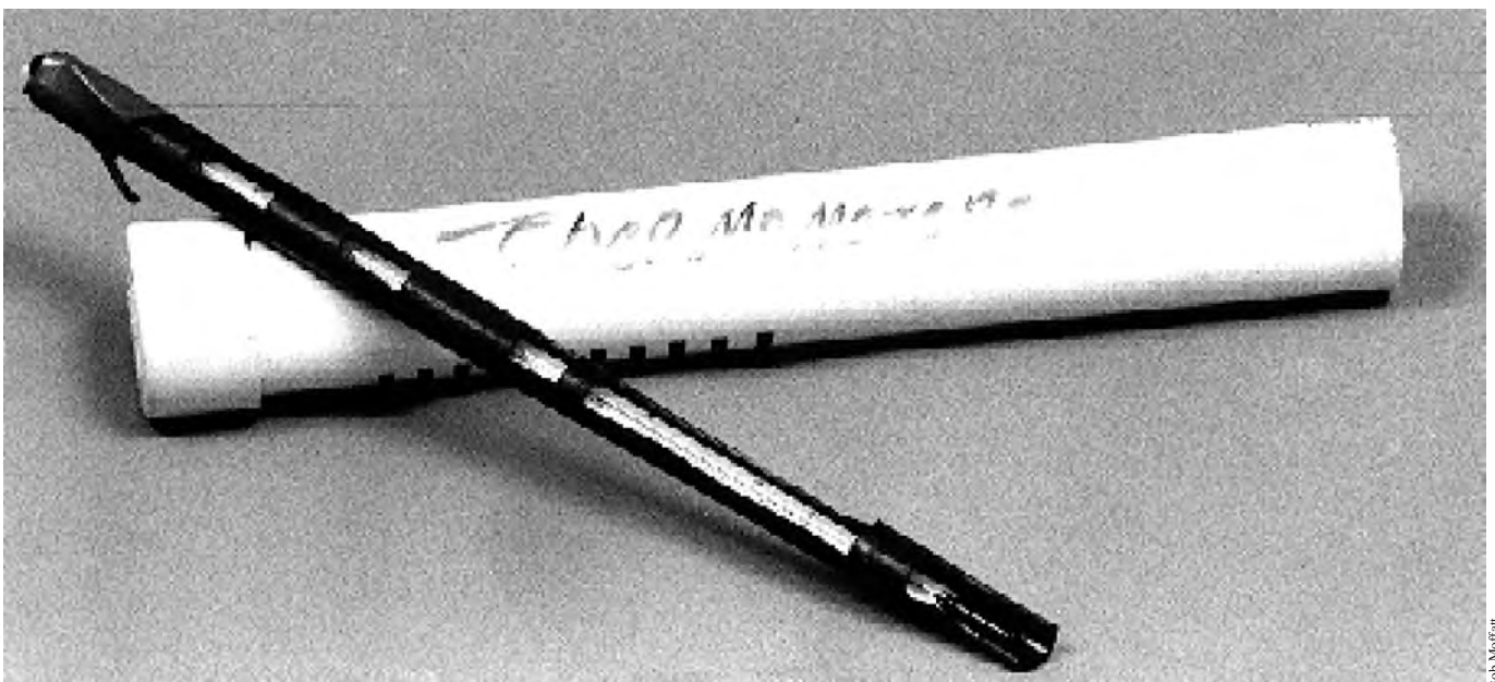
Figure 97.2 Home made field thermometer. A number can be stored in a sink drain pipe with a cap at each end.
